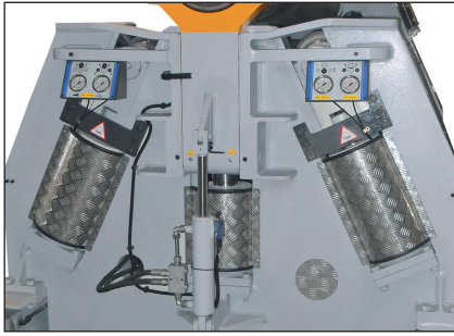
Linear guide system, pistons use all power for bending material
