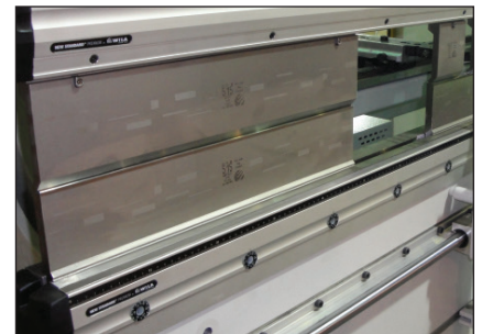
Wila top & bottom hydraulic clamping system
