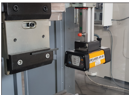
Front laser safety system with safety PLC for CE compatibility
