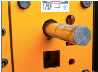
② Steel bar shearing station
