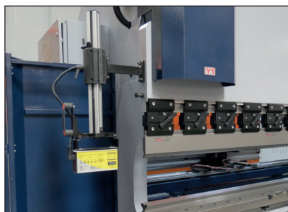
Front laser safety system with safety PLC for CE compatibility
