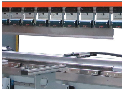
Rolleri top & bottom hydraulic clamping system
